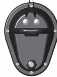
Figure 9 - Apollo 816-1K Series Limit Screw Adjustment
